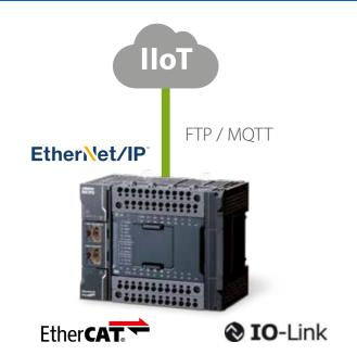
IO-Link provides the controller with production data at sensor level.
