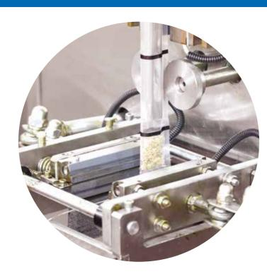
Controlling real sealing temperature guarantees less defects during the sealing process even with thin and eco films
