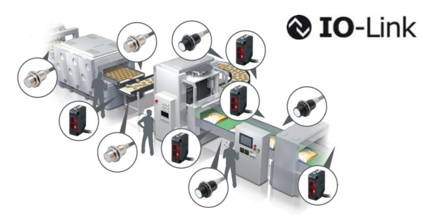
Dynamic configuration thanks to the sensors with IO-Link connectivity.
